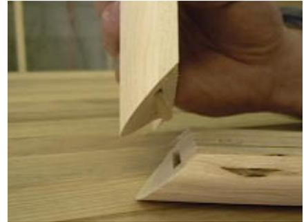
**Figure D - Mitered corners joined together with biscuits**
