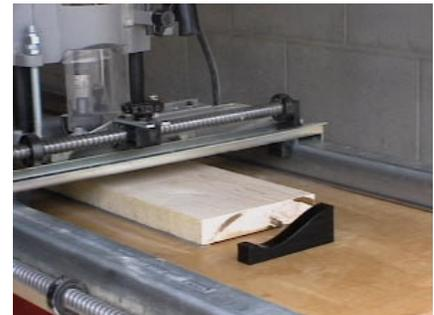
Figure B - End view with bit plunged down onto template
